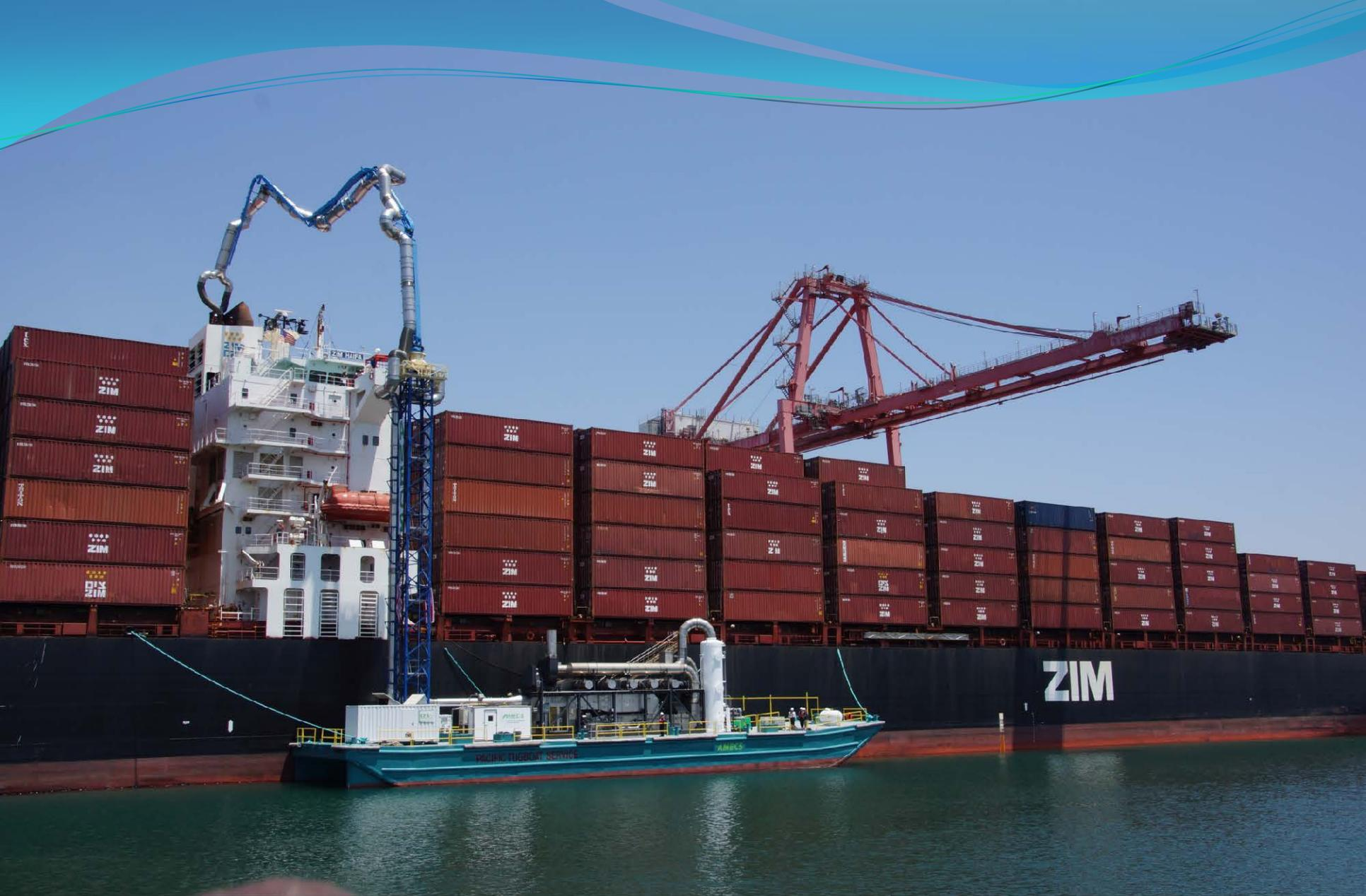
Barge mounted AMECS with a direct connection to the ship's exhaust.
